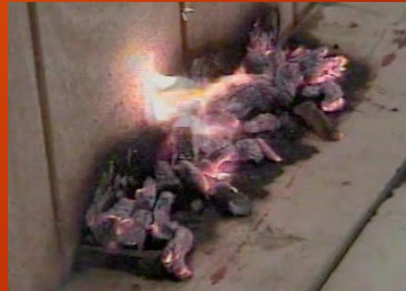
Smoldering/glowing combustion burns surface carbon (char)
